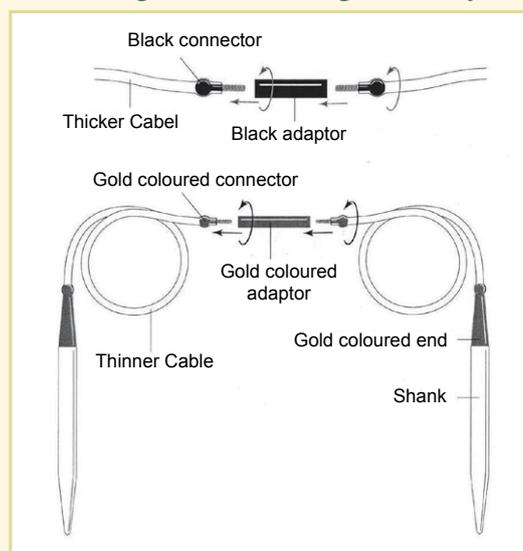
Choose 2 Cables of the Same thickness ( not necessarily the Same length ) and attach ONE end of each cable to your desired Pairs of shanks as illustrated
