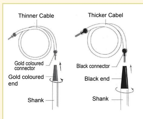
Twist colour coded end of shank on to matching colour connector ( as illustrated above ) at each cable end until fully secure to begin creatively knitting
